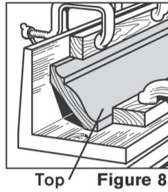
As described, crowns do not lie flush against the wall. Cutting correct 45° mitres is critical. Clamp two blocks of wood to the mitre box to hold the moulding in place at the angle at which it will be installed. Once blocks are in place, insert moulding prior to cutting, face out and upside down (Fig.8). Then cut your 45° angles with a fine tooth saw. To flat cut crown mouldings with a compound mitre saw refer to the owner's manual that came with your saw.
