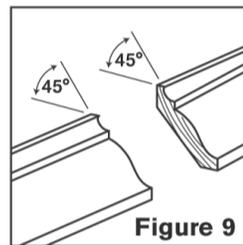
To span longer lengths, you may have to splice your crowns. Set your mouldings in a mitre box or compound mitre saw as described in previous section. Mitre the joining ends at 45° angles from front to back. One piece will overlap the other in a scarf joint. (Fig.9), creating a vertical face seam in the finished installation.
